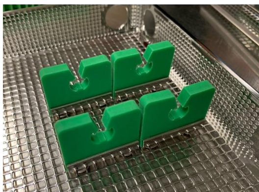
Removable silicone mounts to lock 2 cannulated instruments
